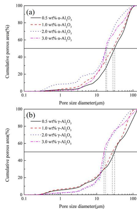
Fig. 2 The cumulative porous area of zircon aggregates with  $\alpha$ - $\text{Al}_2\text{O}_3$  and  $\gamma$ - $\text{Al}_2\text{O}_3$ : (a)  $\alpha$ - $\text{Al}_2\text{O}_3$ ; (b)  $\gamma$ - $\text{Al}_2\text{O}_3$ .
