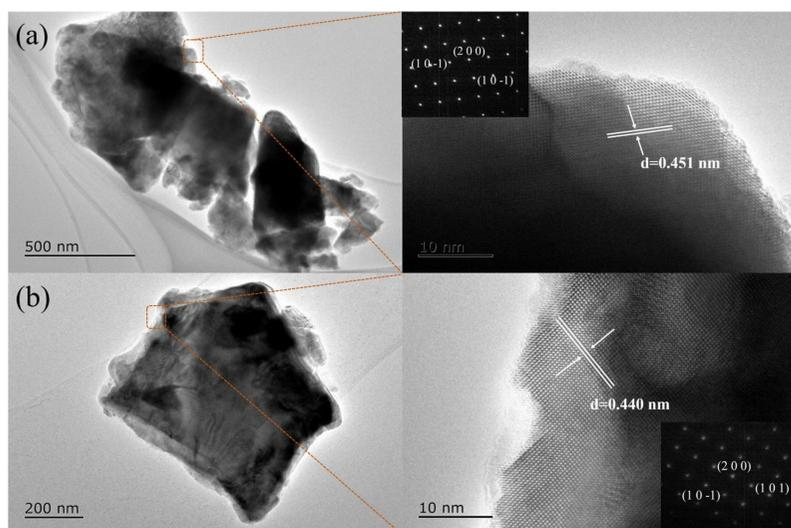
Fig. 1 The TEM images of the samples with different crystal type of  $\text{Al}_2\text{O}_3$ : (a)  $\alpha$ - $\text{Al}_2\text{O}_3$ ; (b)  $\gamma$ - $\text{Al}_2\text{O}_3$ .
